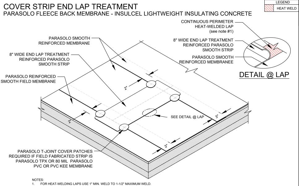
2. REQUIREMENTS AND RECOMMENDATIONS DETAILED IN CURRENT SIPLAST SPECIFICATIONS SHALL APPLY IN ADDITION TO THE ABOVE DRAWING.
