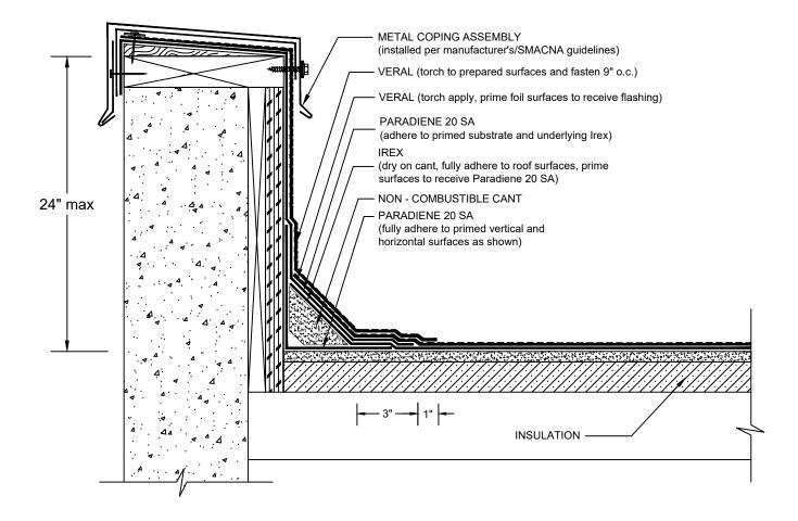
NOTES: 1. WHERE PRIMER IS INDICATED TO MAINTAIN PROPER ADHESION, TA-119 PRIMER IS REQUIRED FOR ALL PARADIENE 20 SA FLASHING REINFORCING AND STRIPPING PLY APPLICATIONS. USE PA-1125 OR PA-917 LS FOR ALL NON-PARADIENE 20 SA APPLICATIONS. CONTACT SIPLAST FOR SPECIFIC REQUIREMENTS.
