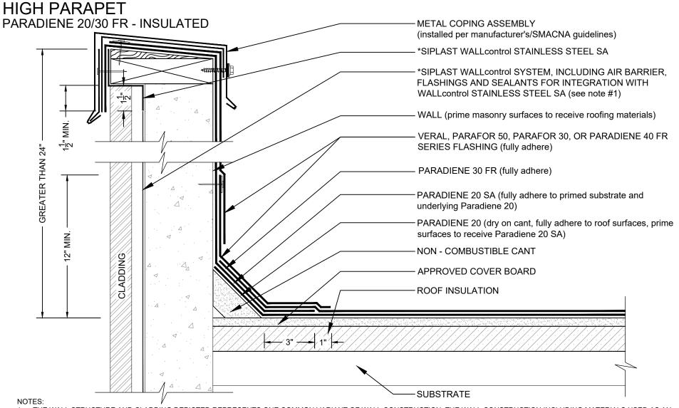
THE WALL STRUCTURE AND CLADDING DEPICTED REPRESENTS ONE COMMON VARIANT OF WALL CONSTRUCTION. THE WALL CONSTRUCTION INCLUDING MATERIALS USED AS AN AIR/MOISTURE BARRIER FOR A SPECIFIC PROJECT MAY DIFFER FROM THAT DEPICTED
