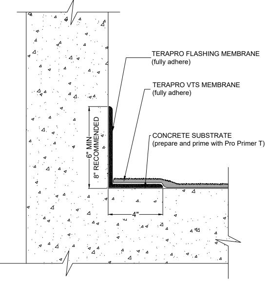
TERAPRO VTS SYSTEM (unreinforced) PRO COLOR FINISH SURFACING AGGREGATE (VTS Quartz) TERAPRO VTS RESIN/FILLER MIXTURE
