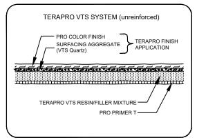
1. REFER TO SIPLAST PREPARATION GUIDELINES FOR PROPER SURFACE PREPARATION OF ALL SUBSTRATES PRIOR TO APPLICATION OF TERAPRO MATERIALS.
