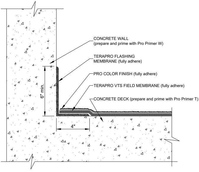
TERAPRO VTS SYSTEM (reinforced) SURFACING AGGREGATE
