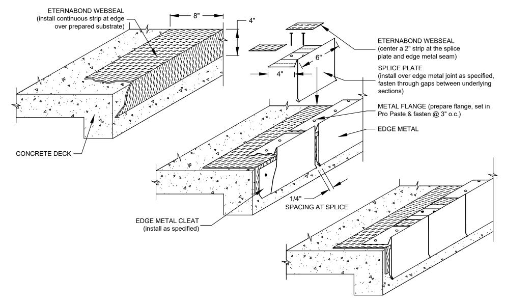
NOTES: 1. REFER TO SIPLAST PREPARATION GUIDELINES FOR PROPER SURFACE TREATMENT OF ALL MATERIALS PRIOR TO APPLICATION OF TERAPRO MATERIALS
