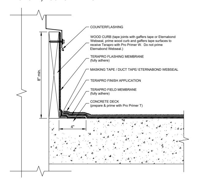
2. REQUIREMENTS AND RECOMMENDATIONS DETAILED IN TERAPRO INSTALLATION SPECIFICATIONS SHALL APPLY IN ADDITION TO THE ABOVE DRAWING.
