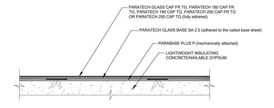
NOTES: 1. REQUIREMENTS AND RECOMMENDATIONS DETAILED IN SIPLAST SPECIFICATIONS SHALL APPLY IN ADDITION TO THE ABOVE DRAWING.
