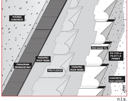
SLOPE 0" - 1/2" per ft\* MATERIALS per 100 sq ft PA-1125 OR PA-917 LS PRIMER 1 gal 73 lbs **PRO BASE TG** PARARO ROOF RESIN 19 kg **PRO FLEECE** PARAPRO ROOF RESIN 12 kg PARADRAIN DRAINAGE MAT 25 lbs **CONCRETE SURFACING**
