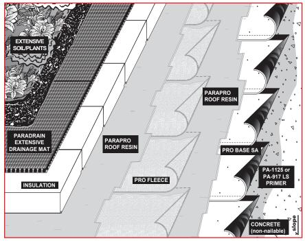
SLOPE 0" to 1" per foot min.\* **MATERIALS** per 100 sq ft PA-1125 OR PA-917 LS PRIMER 1 gal **PRO BASE SA** 69 lb PARAPRO ROOF RESIN 19 kg **PRO FLEECE** PARAPRO ROOF RESIN 12 kg **XPS INSULATION** PARADRAIN EXTENSIVE 25 lb **DRAINAGE MAT** SOIL/PLANTS
