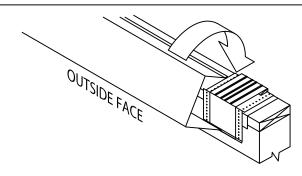
STEP 9 - COPING HOOK OUTSIDE FACE OF COPING OVER THE ANCHOR CLIPS AND ROTATE INTO PLACE. ENGAGE REAR LEG ONTO ANCHOR CLIPS BY PRESSING DOWNWARD UNTIL SNAP LOCK OCCURS.
