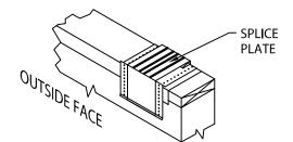
STEP 8 - SPLICE PLATES PLACE SPLICE PLATE ONTO ANCHOR CLIPS AT SPLICE JOINTS, 12'-0" O.C. NOTE: REMOVE RELEASE PAPER FROM SEALANT STRIPS.
