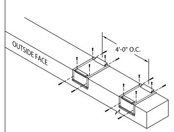
STEP 7 - ANCHOR CLIPS LOCATE OVER MEMBRANE AND FASTEN GALVANIZED ANCHOR CLIPS TO WALL AT 4'-0" CENTER WITH PROVIDED FASTENERS AS SHOWN IN DETAIL A.
