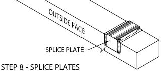
PLACE SPLICE PLATE ONTO ANCHOR CLIPS AT SPLICE JOINTS, 12'-0" O.C.
