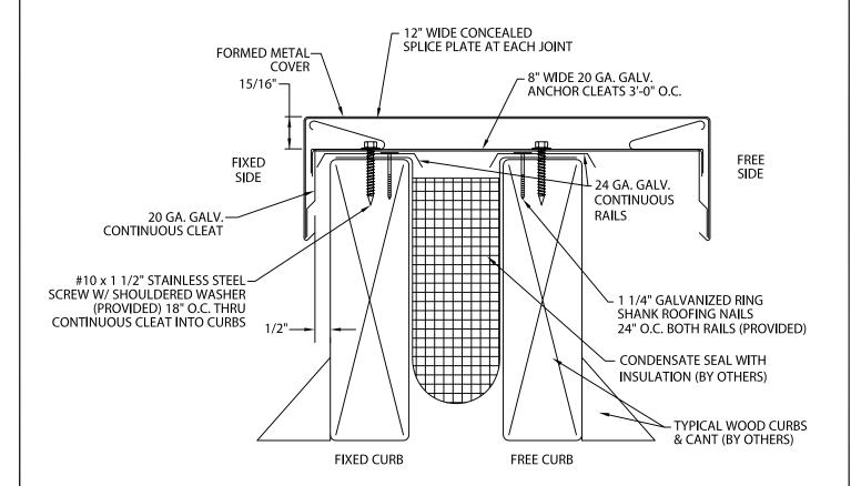
NOTE: REFERENCE THE SIPLAST PARAGUARD ROOF TO WALL EXPANSION JOINT DETAIL FOR THE APPROVED MEMBRANE PLY CONFIGURATION AND APPROVED COUNTER FLASHING METHOD.
