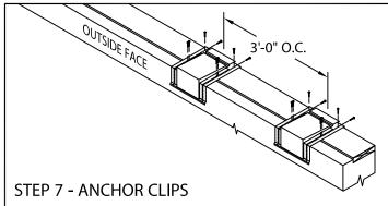
LOCATE AND FASTEN GALVANIZED ANCHOR CLIPS TO WALL AT 3'-0" CENTERS WITH PROVIDED FASTENERS FOR SUBSTRATE (SEE DETAIL A).
