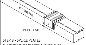
PLACE SPLICE PLATE ONTO ANCHOR CLIPS AT SPLICE JOINTS, 12'-0" O.C. NOTE: REMOVE RELEASE PAPER FROM SEALANT STRIPS.
