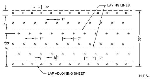
NOTES: 1. THE ABOVE FASTENING PATTERNS ARE RECOMMENDED FOR BASE SHEET SECUREMENT BELOW SIPLAST MEMBRANE SYSTEMS.
