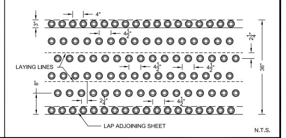
NOTES: 1. THE ABOVE FASTENING PATTERNS ARE RECOMMENDED FOR BASE SHEET SECUREMENT BELOW SIPLAST MEMBRANE SYSTEMS.
