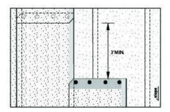
Fasten the finish ply with roofing screws and 2-inch metal plates. Each head lap should be fastened using four fasteners evenly spaced from side lap to side lap. All fasteners should be covered by a succeeding ply extending a minimum of 3 inches beyond the lowermost edge of the fastener caps.
