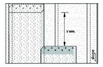
Fasten the finish ply with nails having attached caps of a minimum of 1-inch diameter. Each head lap should be fastened using nine nails in a double row, evenly spaced configuration. Stagger the rows of nails. All fasteners should be covered by a succeeding ply extending a minimum of 3 inches beyond the lowermost edge of the fastener caps.
