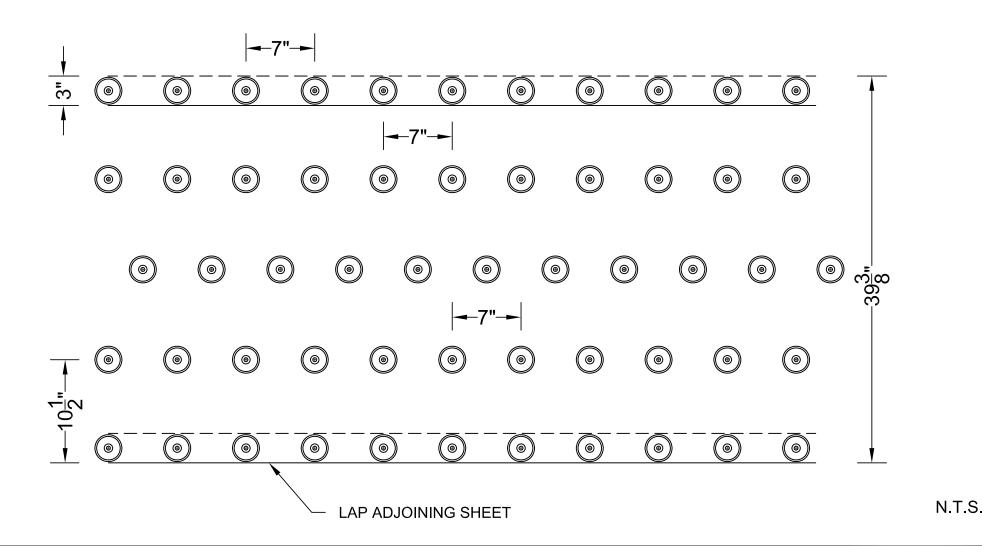
NOTES: 1. THE ABOVE FASTENING PATTERNS ARE RECOMMENDED FOR BASE SHEET SECUREMENT BELOW SIPLAST MEMBRANE SYSTEMS.
