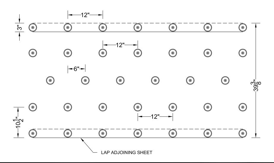
NOTES: 1. THE ABOVE FASTENING PATTERNS ARE RECOMMENDED FOR BASE SHEET SECUREMENT BELOW SIPLAST MEMBRANE SYSTEMS.
