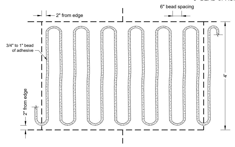
NOTES: 1. THE ABOVE BEAD SPACING FREQUENCY IS INTENDED AS A GUIDELINE FOR INSULATION ADHESION BELOW SIPLAST MEMBRANE SYSTEMS AND IS SUBJECT TO SIPLAST AND INDUSTRY STANDARD REQUIREMENTS.
