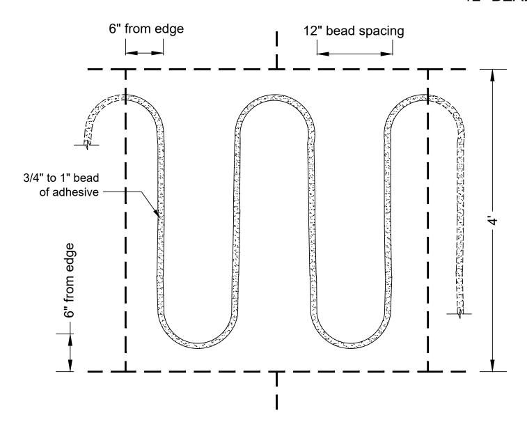
NOTES: 1. THE ABOVE BEAD SPACING FREQUENCY IS INTENDED AS A GUIDELINE FOR INSULATION ADHESION BELOW SIPLAST MEMBRANE SYSTEMS AND IS SUBJECT TO SIPLAST AND INDUSTRY STANDARD REQUIREMENTS
