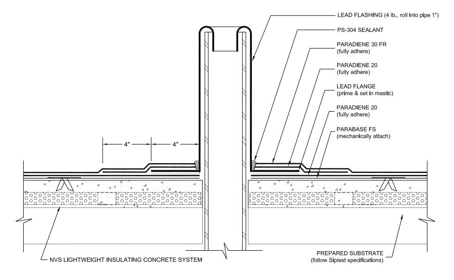
NOTES: 1. WHERE PRIMER IS INDICATED TO MAINTAIN PROPER ADHESION, TA-119 PRIMER IS REQUIRED FOR ALL PARADIENE 20 SA FLASHING REINFORCING AND STRIPPING PLY APPLICATIONS. USE PA-1125 OR PA-917 LS FOR ALL NON-PARADIENE 20 SA APPLICATIONS. CONTACT SIPLAST FOR SPECIFIC REQUIREMENTS.
