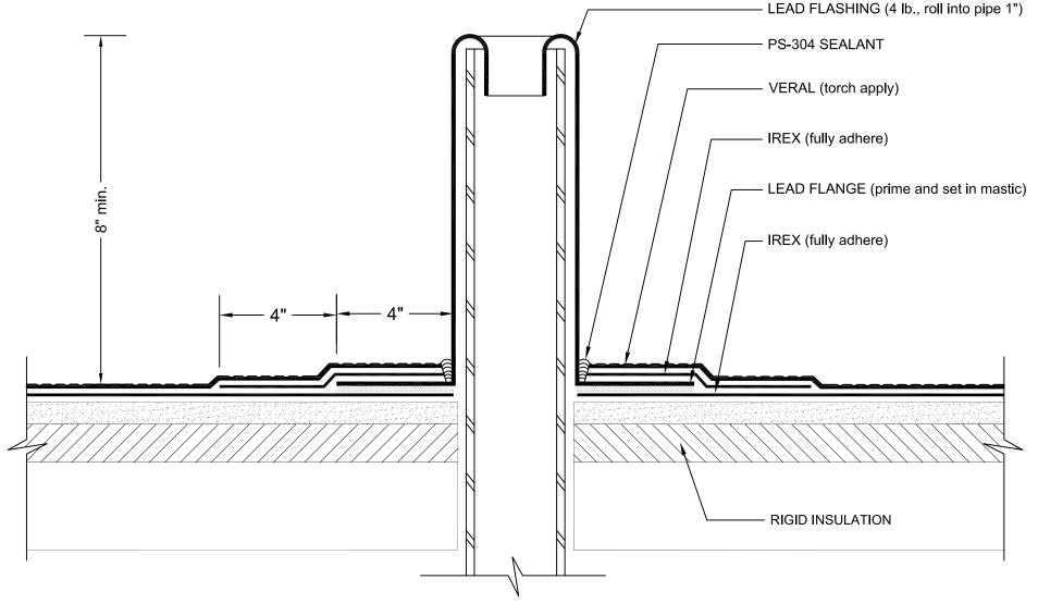
NOTES: 1. WHERE PRIMER IS INDICATED TO MAINTAIN PROPER ADHESION, TA-119 PRIMER IS REQUIRED FOR ALL PARADIENE 20 SA FLASHING REINFORCING AND STRIPPING PLY APPLICATIONS. USE PA-1125 OR PA-917 LS FOR ALL NON-PARADIENE 20 SA APPLICATIONS. CONTACT SIPLAST FOR SPECIFIC REQUIREMENTS.
