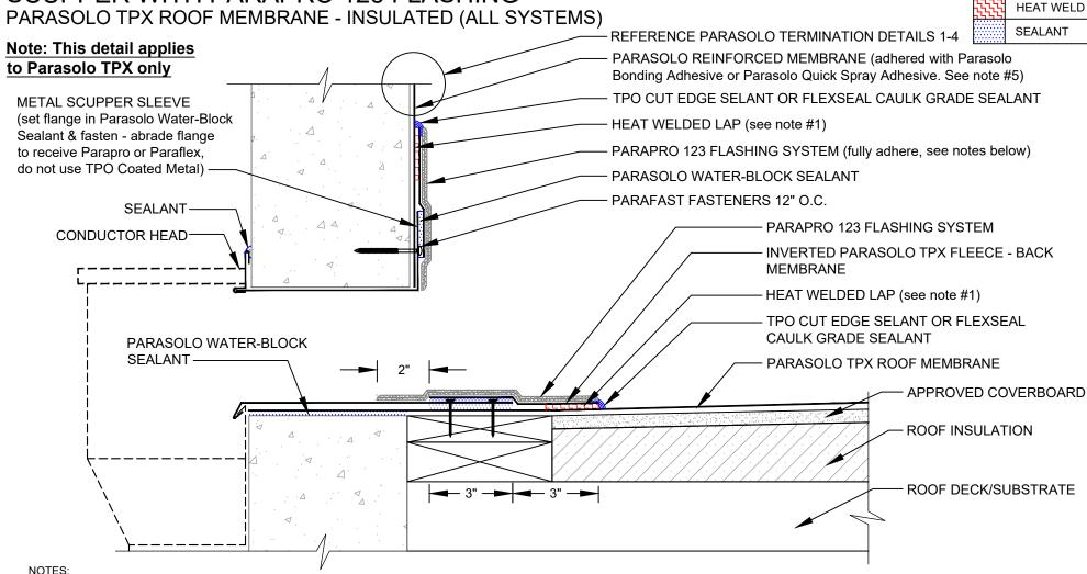
FOR HEAT-WELDING LAPS USE 1" MINIMUM TO 1-1/2" MAXIMUM WELD.
