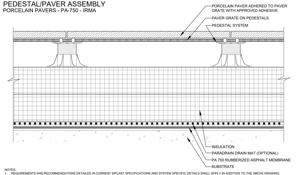
DESIGNER OF RECORD TO VERIFY CAPACITY OF DECK/SUBSTRATE TO ACCOMMODATE LOAD OF THE OVERBURDEN COMPONENTS.
