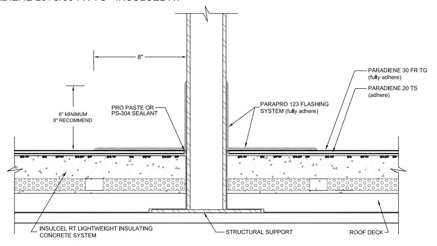
NOTES: 1. BEFORE APPLICATION OF THE PARAPRO FLASHING MEMBRANE, PRO PASTE, OR PS-304 ELASTOMERIC SEALANT SHOULD BE USED TO FILL VOIDS WHERE ROOFING MEMBRANES TERMINATE AT PENETRATIONS.
