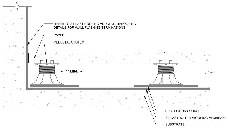
REQUIREMENTS AND RECOMMENDATIONS DETAILED IN CURRENT SIPLAST SPECIFICATIONS AND SYSTEM SPECIFIC DETAILS SHALL APPLY IN ADDITION TO THE ABOVE DRAWING
