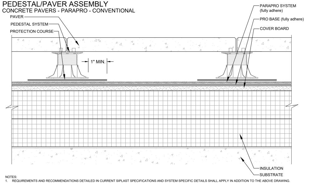
DESIGNER OF RECORD TO VERIFY CAPACITY OF DECK/SUBSTRATE TO ACCOMMODATE LOAD OF THE OVERBURDEN COMPONENTS.
