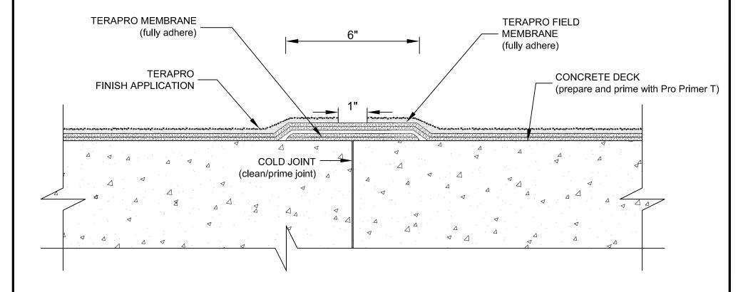
NOTES: 1. REFER TO SIPLAST PREPARATION GUIDELINES FOR PROPER SURFACE TREATMENT OF ALL MATERIALS PRIOR TO APPLICATION OF TERAPRO MATERIAL.
