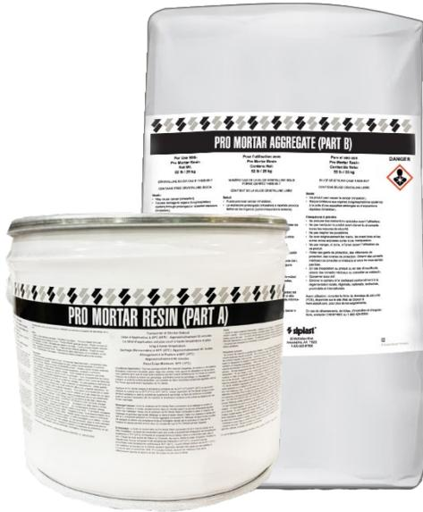
Pro Mortar is a multi-component, fast curing, PMMA resin-based mortar consisting of Pro Mortar Resin (Part A), a PMMA resin, and Pro Mortar Aggregate (Part B). One pail of Pro Mortar Resin (Part A) is mixed with two bags of Pro Mortar Aggregate (Part B) and the mixture is then catalyzed with four bags of Pro Catalyst to initiate cure.
