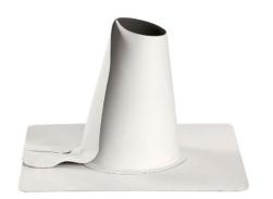
Parasolo PVC Split Pipe Boots are factory formed and fabricated from reinforced Parasolo PVC and are used for flashing round and conical penetrations. Split boots can be used to flash penetrations that cannot be overlaid with a closed boot. Boots include a stainless steel clamp to facilitate termination at the top of the boot. Three sizes are available: 1"-2", 3"-5" and 6"-8".
