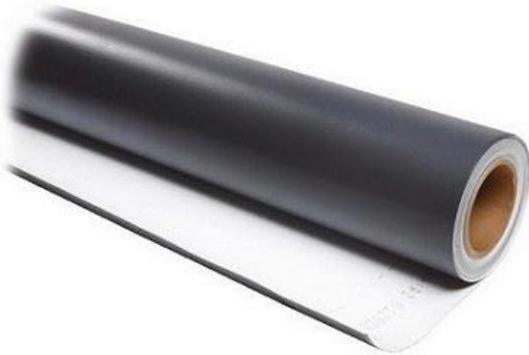
Parasolo® KEE is a single-ply membrane utilizing a PVC blend with DuPont's™ Elvaloy® Ketone Ethylene Ester (KEE) solid-phase flexibilizer and non-wicking polyester scrim reinforcement. Parasolo KEE is heat weldable and has excellent fire and chemical resistance properties.
