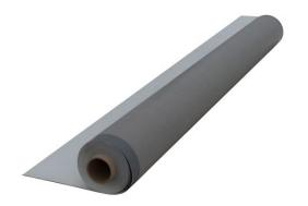
Parasolo® KEE is a single-ply membrane utilizing a PVC blend with DuPont's™ Elvaloy® Ketone Ethylene Ester (KEE) solid-phase flexibilizer and non-wicking polyester scrim reinforcement manufactured at a minimum thickness. Parasolo KEE Fleece-Back is heat weldable and has excellent fire and chemical resistance properties.
