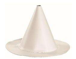
Parasolo PVC Conical Pipe Boots are factory formed from unreinforced PVC and are used for flashing cylindrical and conical penetrations. Boots include a stainless steel clamp to facilitate termination at the top of the boot.
