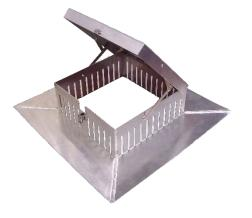
ParaGREEN<sup>™</sup> Drain Chamber is designed to work with all Siplast vegetated roof systems and fits over the standard internal roof drain assembly. It isolates green roof components, ballast and debris from the immediate drain area and facilitates drainage from the field of the vegetated roof assembly to the internal drain. The hinged cover allows for easy maintenance access.
