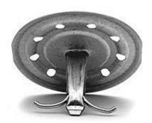
Parafast® Twin-Loc Fasteners are factory preassembled units consisting of a tube, integral disk, and locking staple. The tube is fabricated from coated steel, the 2.7-inch disk is ribbed and is fabricated from coated steel, and the locking staple is fabricated from coated high-tensile steel wire. Parafast Twin-Loc Fasteners are designed to secure base sheets in approved assemblies to approved substrates.
