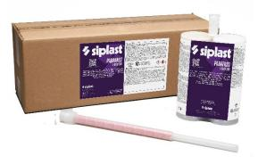
Parafast<sup>®</sup> 1-Step LRF Cartridge is an elastomeric, all-purpose, foamable adhesive used for adhering rigid insulation boards to substrates approved in advance by Siplast. Designed to be used in one step, Parafast 1-Step LRF Cartridge provides a quick application by eliminating the need for mixing, pump carts, or spray rigs. It has no temperature application restrictions and offers a quick set time.
