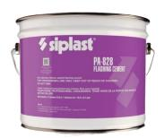
PA-828® Flashing Cement is specially formulated cold process winter grade adhesive designed for use as a roofing membrane flashing cement. PA-828 Flashing Cement is a slump-resistant asphalt cutback adhesive for high slope and vertical applications. It is designed for use with guaranteed Siplast Roof Systems as a membrane flashing adhesive for granule surfaced styrene-butadiene-styrene (SBS) sheets.
