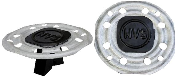
The Siplast NVS Fastener is formed from specially coated galvanized steel. The split-wedge leg spreads upon installation into lightweight insulating concrete to provide withdrawal resistance. NVS Fasteners are assembled to incorporate a corrosion resistant Galvalume<sup>®</sup> coated stress distribution plate.
