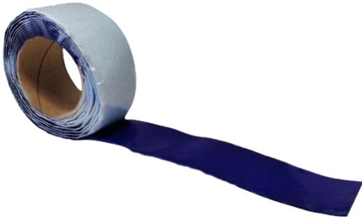
Monarflex® Blue Monobond is a permanently flexible butyl-based joint tape for use with Monarflex Scaffold Sheeting. This double-sided, self-adhesive tape provides a seal where two sheeting sections overlap. The adhesive used on Blue Monobond is comprised of a butyl-based, non-hardening, permanently flexible, high-performance sealant.
