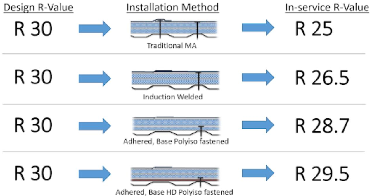
*Figure showing In-Service R-value based on modeling a 15,000 square foot roof with a 120mph wind speed used to determine the fasteners quantities and densities.*
