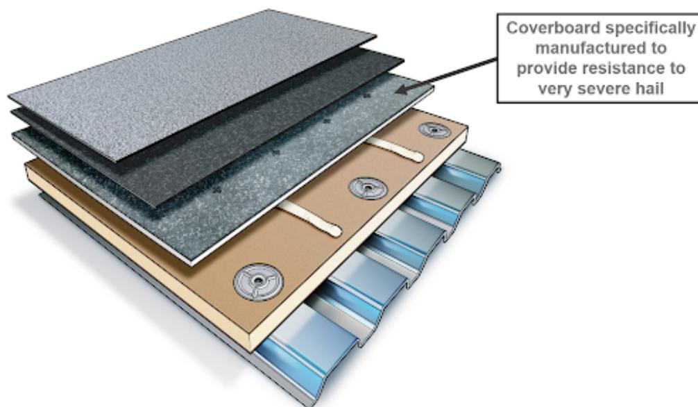
*Figure showing a coverboard specifically manufactured to provide resistance to very severe hail*
