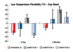
very quickly. Two sheets of different thicknesses, manufactured with the same blend, will not pass at the same temperature. The thicker sheet will fail first because the stress applied when bending around the test mandrel will be greater.
