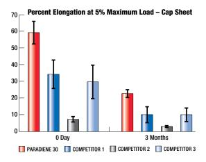
As such, ultimate elongation is the clearest mechanical measure of aging and performance of the elastomeric asphalt/polymer modified blend.
