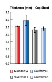
In general, if blend quality is good, performance properties of SBS-modified bitumen membranes are related to the thickness of the blend in the product. While total thickness is important, it is the thickness of the blend, not the thickness of the reinforcing mat or surfacing, that counts. Further, no thickness will make up for a poor quality blend.
