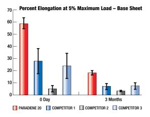
Ultimate elongation is a definitive measure of the elongation of the SBS blend, not the elongation of the glass reinforcement. As the graphs show, some materials have elongation values no better than those of the reinforcing material. Ultimate elongation is directly related to the integrity of the SBS-modified bitumen.
