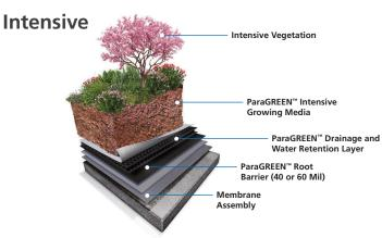
ParaGREEN<sup>™</sup> Intensive layered vegetated roof assemblies incorporate deeper media depths, typically ≥ 12 in. supporting a wide range of plant material. ParaGREEN<sup>™</sup> Intensive solutions are employed in applications from amenity decks to immersive landscapes on podium.
