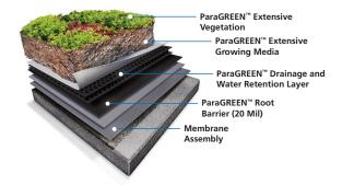
ParaGREEN<sup>™</sup> Extensive layered vegetated roof assemblies incorporate shallower media depths commonly ranging from 3 in. – 8 in. and can be tailored to fit within project thresholds. ParaGREEN<sup>™</sup> Extensive can be planted with ParaGREEN<sup>™</sup> Vegetated Mats or containerized herbaceous plants.
