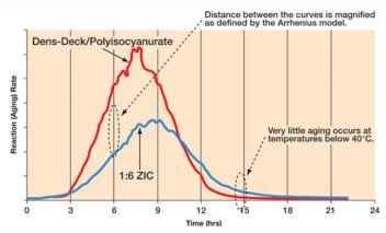
At each of the circled locations, where the curves display a membrane temperature difference of 18°F (10°C), the membrane aging rate doubles, as defined by the Arrhenius Equation.
