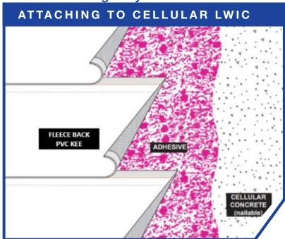
In most cases, Single Ply roofs are adhered using a spatter pattern of low rise foam or bonding adhesives to the substrate. The Single Ply membrane used for this application is most commonly a fleece-back membrane, but smooth back is becoming more frequent in this application.
