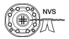
NVS is designed for re-roof applications and has a topping thickness of **1** inch over the Insulperm, and a 1-inch NVS fastener is specifically required.
