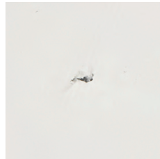
Damaged/punctured Parasolo membrane.
