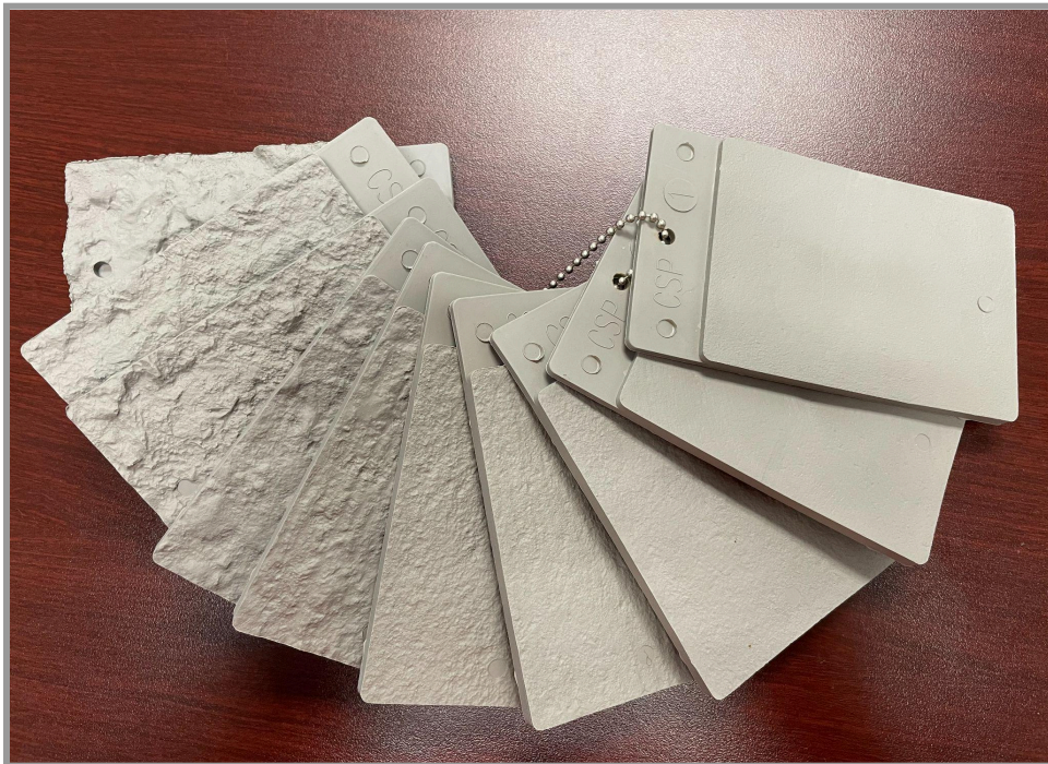
Figure 1: Photo showing physical samples of Concrete Surface Profiles 1 through 10 (R to L) as developed by the International Concrete Repair Institute
