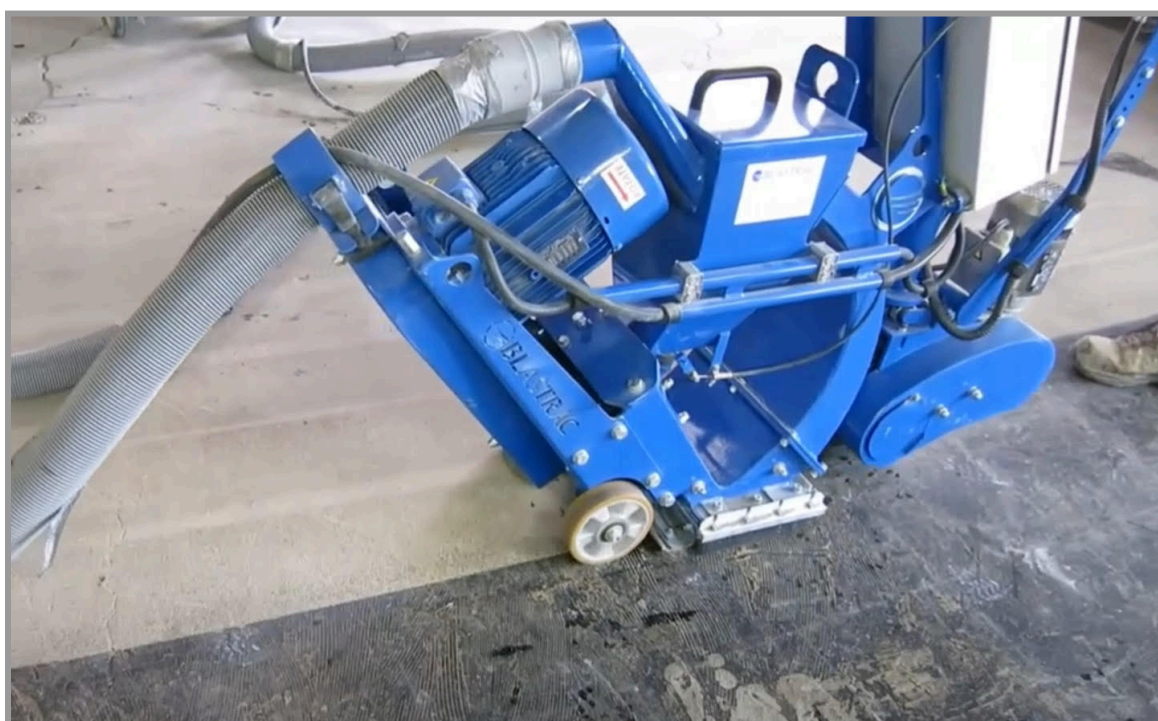
Figure 6: A photo of equipment used to shot blast a concrete roof deck
